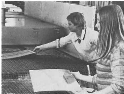
By changing from fuel fired to electric infrared the drying time of name plates is reduced from 40 minutes to 4 minutes.
